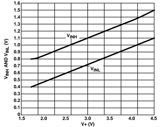
FIGURE 18. DIGITAL SWITCHING POINT vs SUPPLY VOLTAGE
