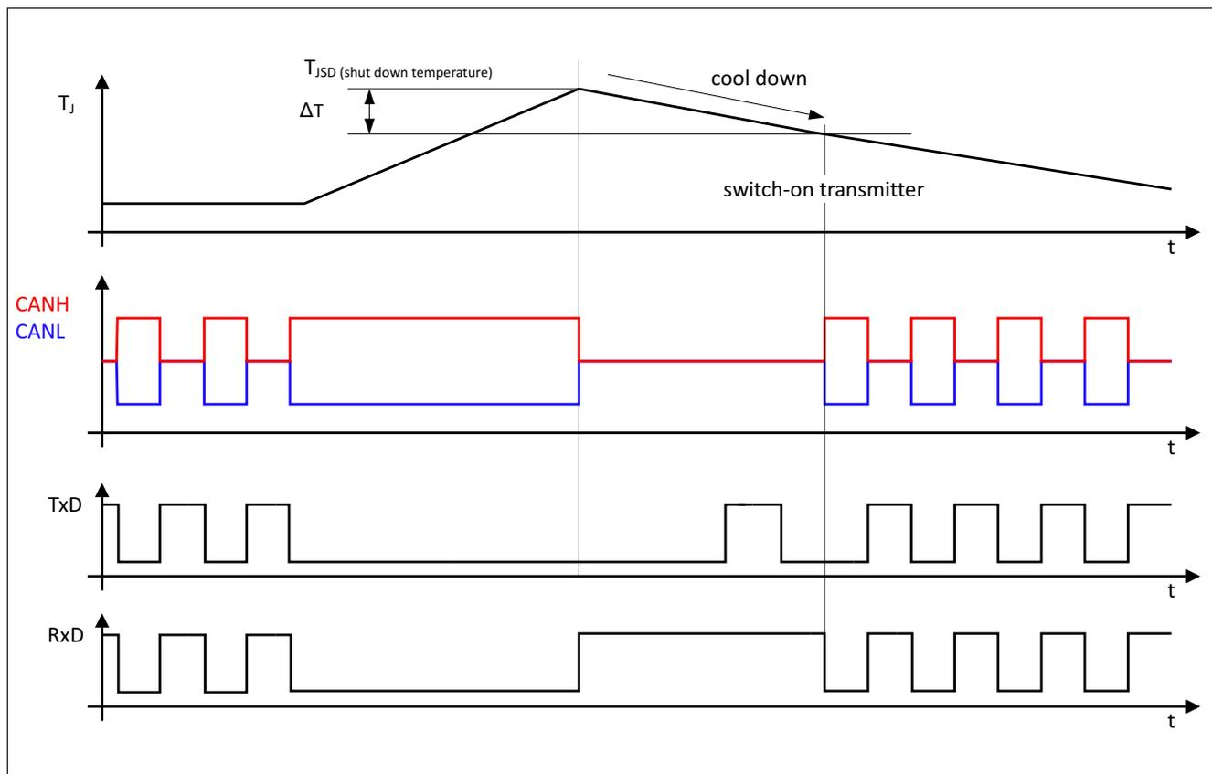
Figure 9 Overtemperature protection
