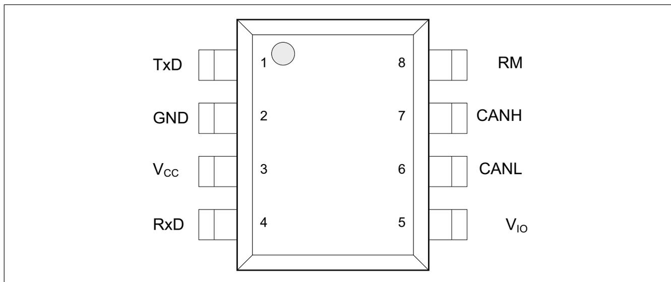
Figure 2 Pin configuration
