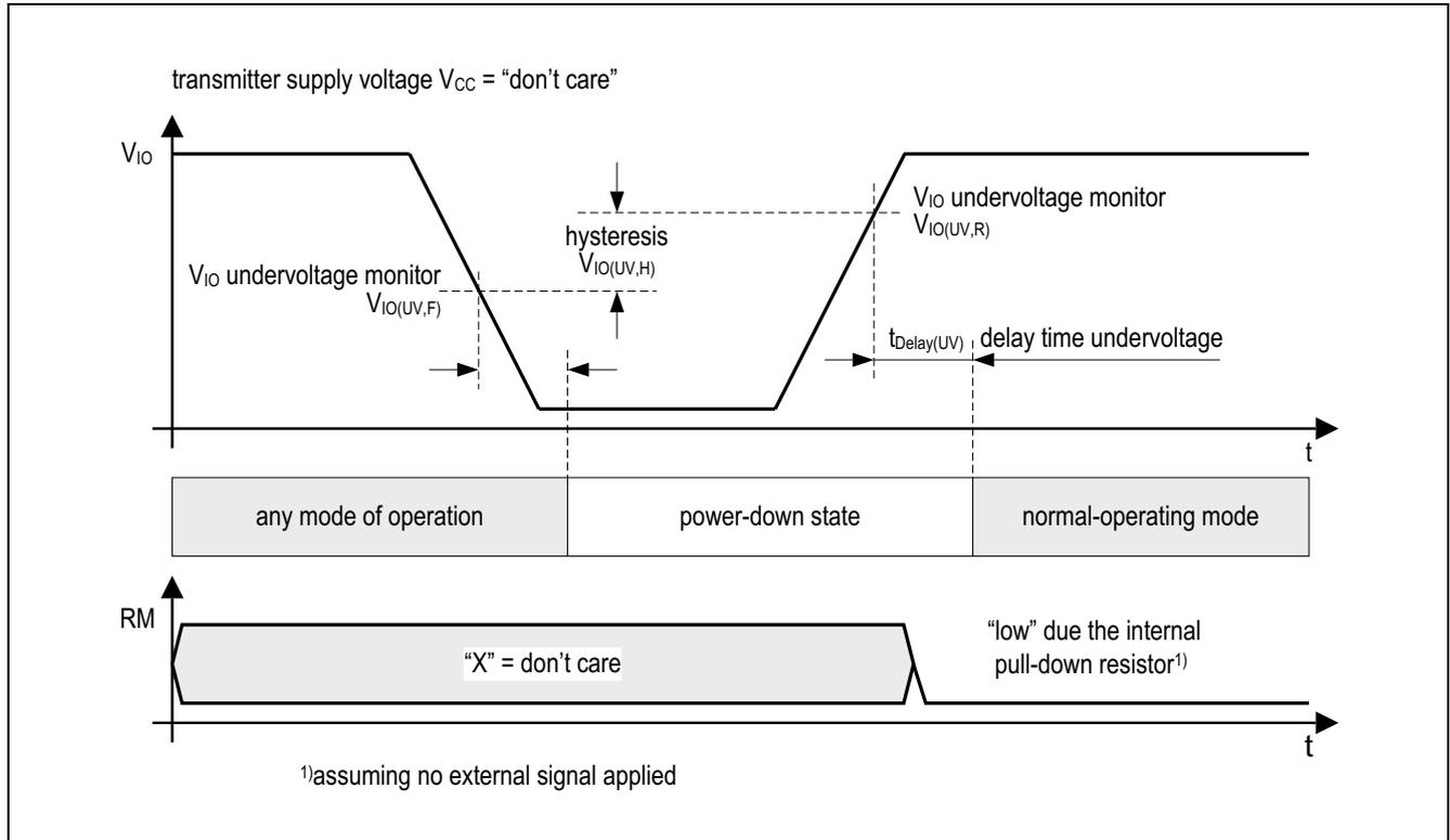
Figure 6 Undervoltage on the digital supply  $V_{IO}$
