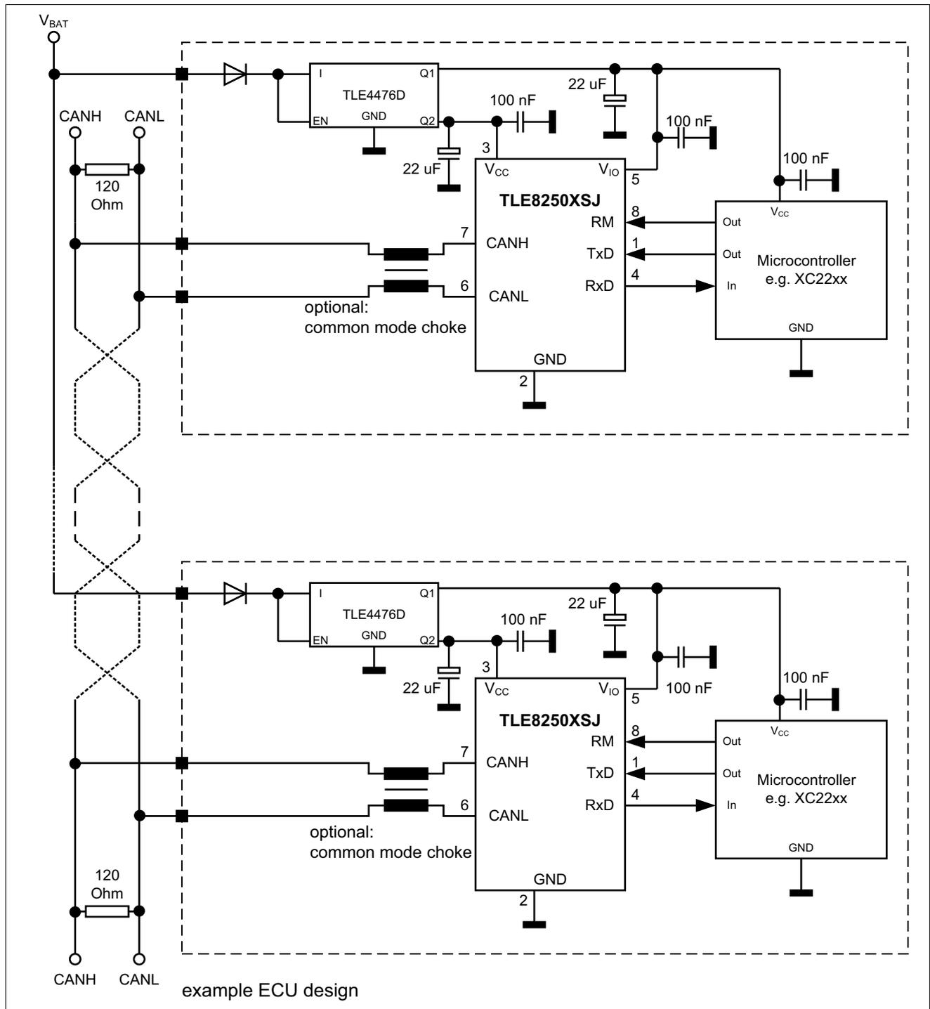
Figure 13 Application circuit
