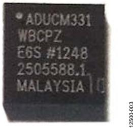
Figure 3. ADuCM331 Device Orientation
