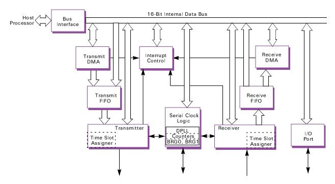
The on-chip DMA channels allow high speed data transfers for both the receiver and the transmitter. The IUSC supports automatic status and control transfer through DMA, and allows initialization of the serial controller under DMA control. Each DMA channel can do a 16-bit transfer in as little as three 50 ns clock cycles, and can generate addresses compatible with 32-, 24- or 16-bit memory ranges.
