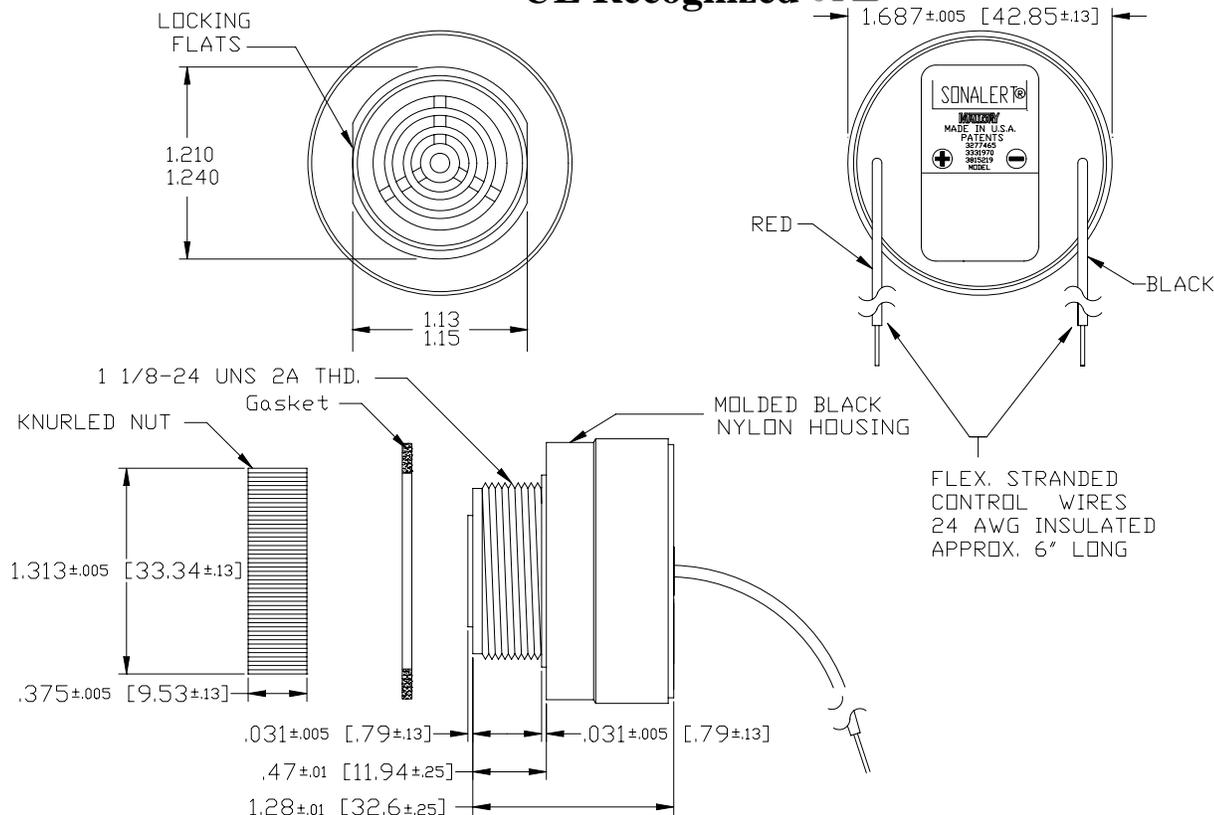
NOTE A: MOUNTING- REMOVE BLACK PLASTIC NUT WHILE LEAVING GASKET ON THREADED NECK OF ALARM. INSERT THREADED NECK THROUGH APPROPRIATE SIZED PANEL HOLE. SCREW NUT BACK ONTO THREADED FRONT SECURING ALARM TO PANEL. MAX RECOMMENDED TORQUE IS 10 IN-LBS.
