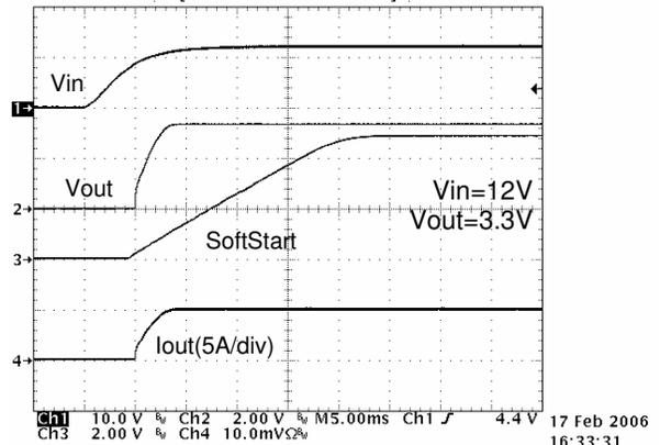
**Figure 6. Start-Up Response: 5A Load**
