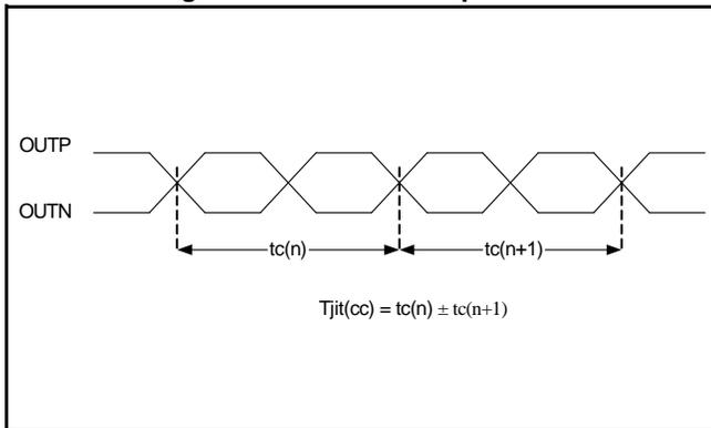
Figure 3: Cycle-cycle jitter
