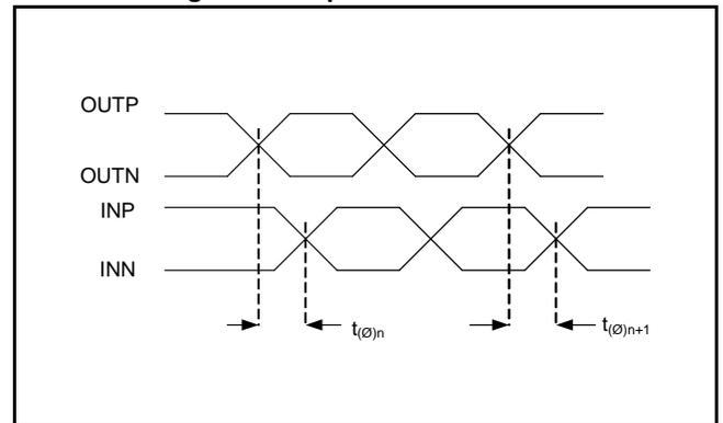
Figure 4: Static phase offset (from input to output)
