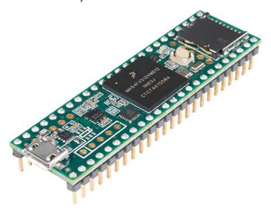
**Description:** The Teensy is a breadboard-friendly development board with loads of features in a, well, teensy package. Each Teensy 3.5 comes with headers already attached and pre-flashed with a bootloader so you can program it using the onboard USB connection; no external programmer needed! You can program for the Teensy in your favorite program editor using C, or you can install the Teensyduino add-on for the Arduino IDE and write Arduino sketches for it!
