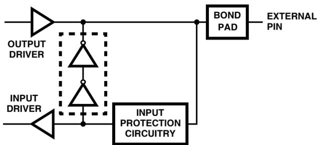
FIGURE 19A. BUS HOLD CIRCUITRY, PINS 36-51, 66, 67
