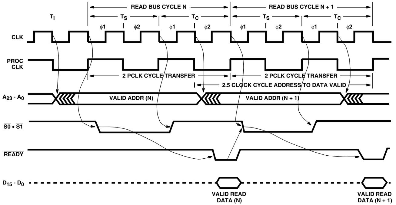
PIPELINED: VALID ADDRESS (N + 1) AVAILABLE IN LAST PHASE OF BUS CYCLE (N).
