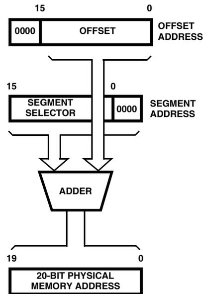
FIGURE 6. 80C286 REAL ADDRESS MODE ADDRESS CALCULATION
