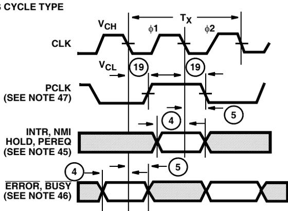
**FIGURE 35. 80C286 ASYNCHRONOUS INPUT SIGNAL TIMING**
