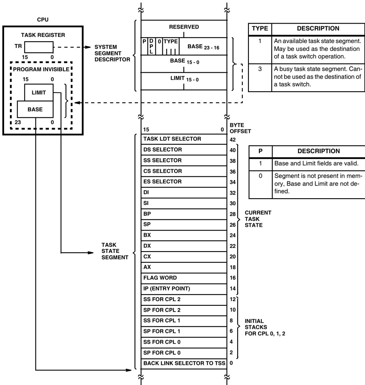
FIGURE 18. TASK STATE SEGMENT AND TSS REGISTERS
