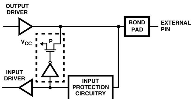
FIGURE 19B. BUS HOLD CIRCUITRY, PINS 4-6, 68
