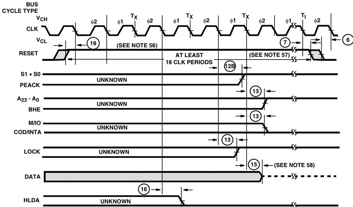
FIGURE 39. INITIAL 80C286 PIN STATE DURING RESET
