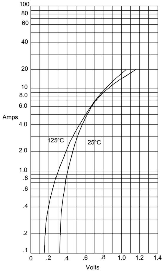
Instantaneous Forward Current - Amperes versus
