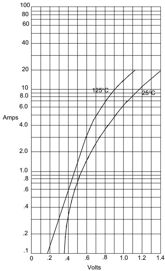
Instantaneous Forward Current - Amperes versus
