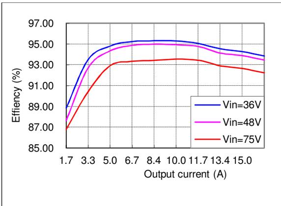
Figure 9: AGF800-48S48P-6L Efficiency Curves @ 25 °C
