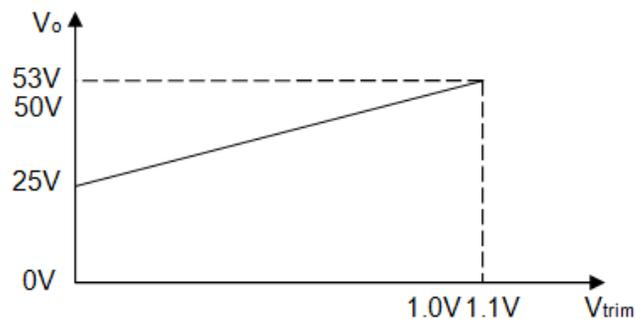
Figure 21  $V_{trim}$  voltage vs. output voltage ( $R_{trim}=5.97k$ )
