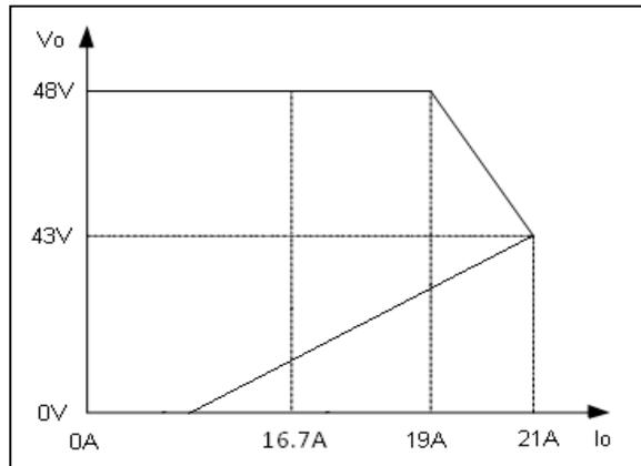
Figure 10: Over-current protection characteristics<sup>1</sup>
