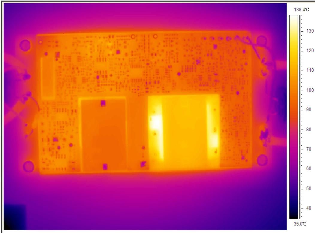
Figure 14 Thermal image, 48V<sub>in</sub>, 48V<sub>o</sub>, full load, room temperature
