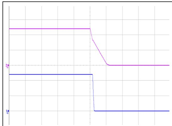
Figure 4: AGF800-48S48P-6L Turn Off Characteristic (100mS/div)
