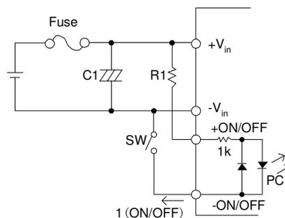
Figure 16 Connection of remote ON/OFF control (A)
