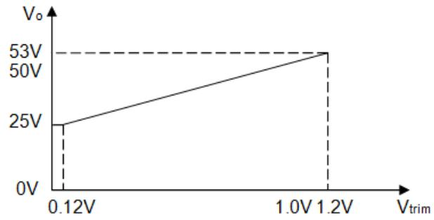
Figure 22  $V_{trim}$  voltage vs. output voltage ( $R_{trim}=5.1k\Omega$ )
