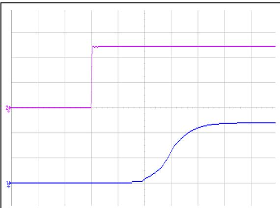
Figure 3: AGF800-48S48P-6L Output Voltage Startup Characteristic (100mS/div)
