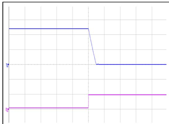
Figure 6: AGF800-48S48P-6L Remote OFF Waveform (20mS/div)
