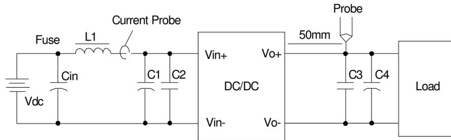
Figure 24 Input ripple & output ripple & noise test configuration
