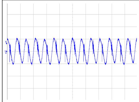
Figure 2: AGF800-48S48P-6L Ripple and Noise Measurement
