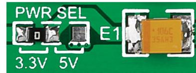
AlphaNum click™ carries a single zero-ohm SMD jumper used to select between 3.3V or 5V I/O voltage levels. The jumper is soldered in the 3.3V position by default.
