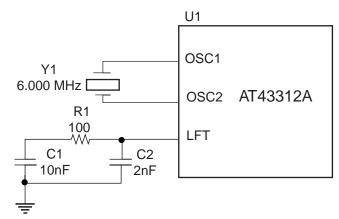
For proper operation of the PLL, an external RC filter consisting of a series RC network of 100 $\Omega$  and 10 nF in parallel with a 2 nF capacitor must be connected from the LFT pin to VSS.
