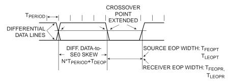
Figure 10. Receiver Jitter Tolerance
