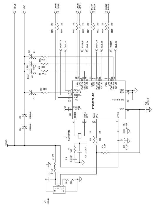
Figure 16. AT43312A Bus-powered USB Hub
