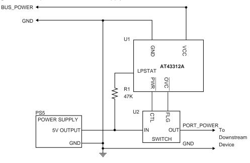
Figure 2. Self-powered Hub Power Supply
