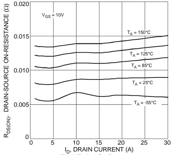
Fig. 7 Typical On-Resistance vs. Drain Current and Temperature
