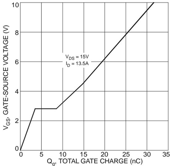
Fig. 14 Gate-Source Voltage vs. Total Gate Charge
