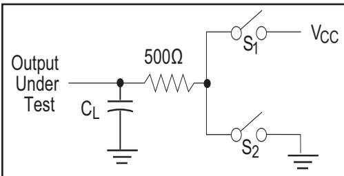
Figure 3. Driver Timing Test Load #2 Circuit
