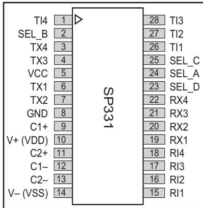
Figure 9. SP331 Pinout
