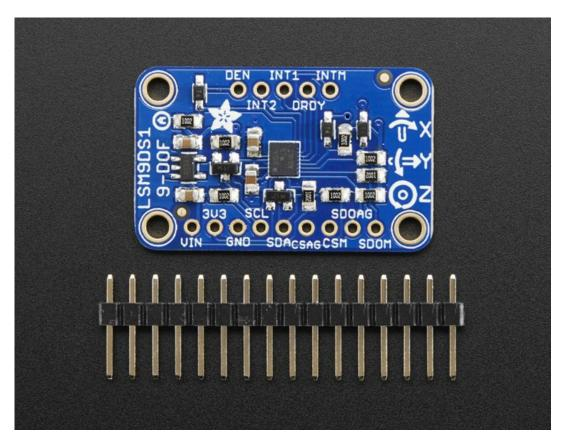
We've carried the LSM9DS0 from ST for a while, and the LSM9DS1 is their latest offering. We thought this could really make for a great breakout, at a very nice price! Design your own activity or motion tracker with all the data... We spun up a breakout board that has all the extra circuitry you'll want, for use with an Arduino (or other microcontroller)
