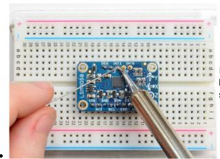
If you plan to use the interrupts and/or you want the board to sit flatter in a breadboard, solder up the other strip!
