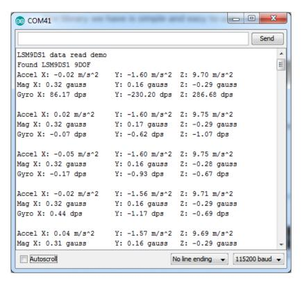
We suggest using this **Adafruit\_Sensor** interface as shown in this demo, since it will let you swap sensors without having to worry about units compatibility. Try twisting and moving the board around to see the sensors change value.
