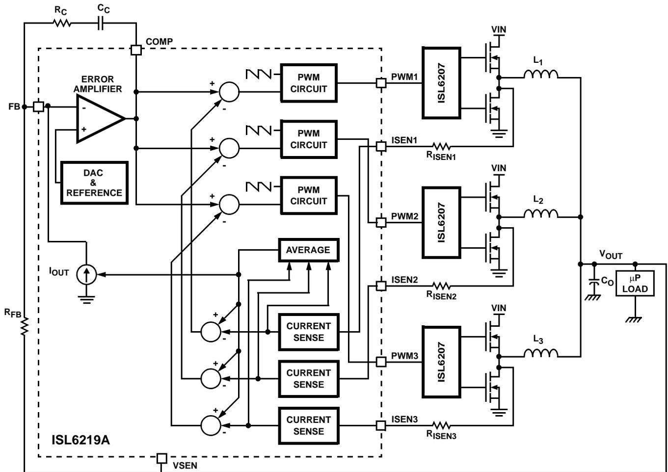
FIGURE 1. SIMPLIFIED BLOCK DIAGRAM OF THE ISL6219A
