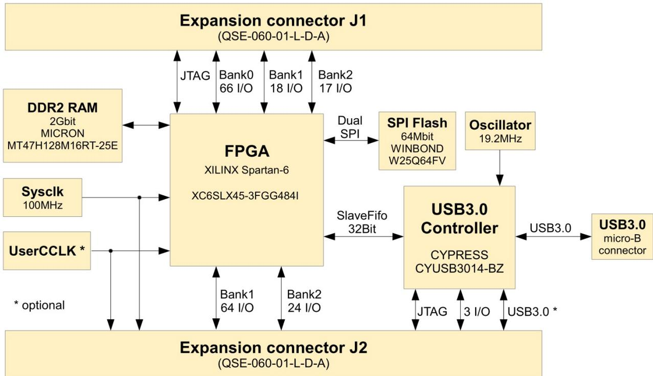
Figure 3: FPGA – USB3 board functional Diagram
