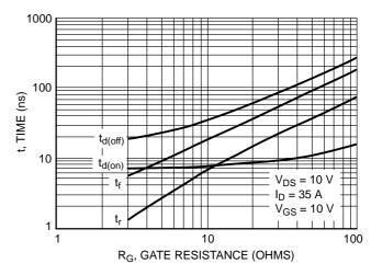
Figure 8. Gate-To-Source and Drain-To-Source
