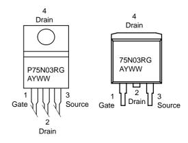
$\begin{array}{lll} xxxxxxx & = Device \ Code \\ G & = Pb-Free \ Device \\ A & = Assembly \ Location \\ Y & = Year \end{array}$
