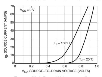
Figure 10. Diode Forward Voltage versus Current
