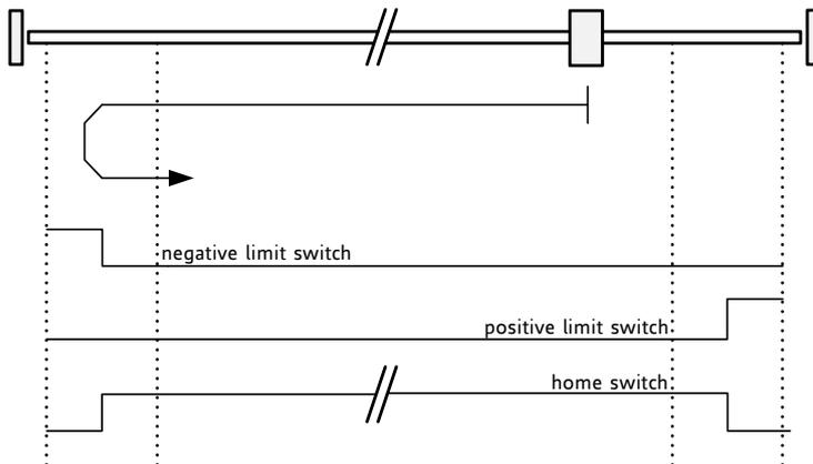
Search home switch in negative direction, reverse the direction when left stop switch reached.
