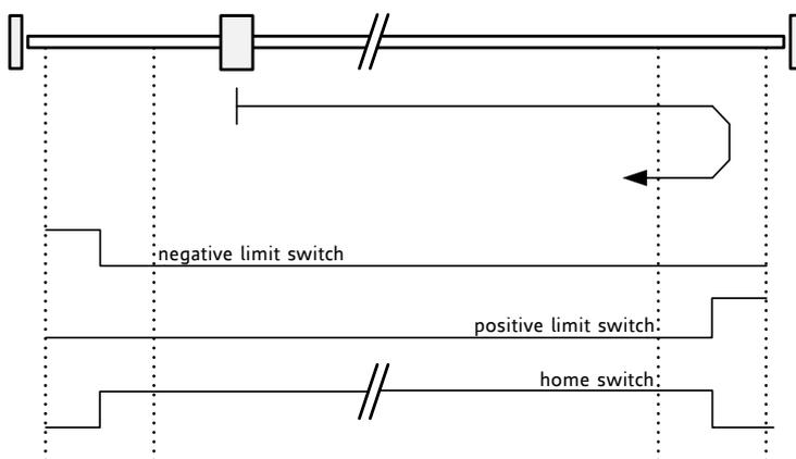
Search home switch in positive direction, reverse the direction when right stop switch reached.
