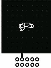
a)  $70^\circ\text{C/W}$  when mounted on a  $1\text{in}^2$  pad of 2 oz copper
