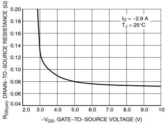
Figure 3. On-Resistance vs. Gate Voltage
