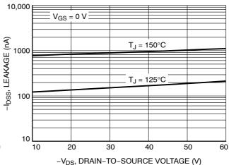
Figure 6. Drain-to-Source Leakage Current vs. Voltage
