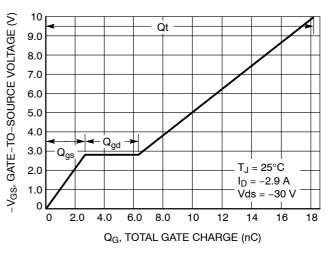
Figure 8. Gate-to-Source Voltage vs. Total Charge
