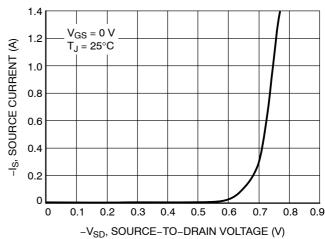
Figure 10. Diode Forward Voltage vs. Current
