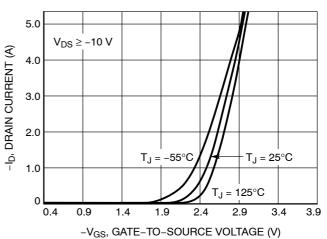
Figure 2. Transfer Characteristics
