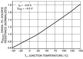
Figure 5. On–Resistance Variation with Temperature
