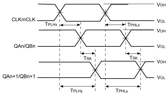
$$T_{SK} = T_{PLHy} - T_{PLHx} \text{ or } T_{SK} = T_{PHLy} - T_{PHLx}$$
