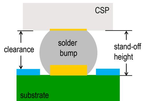
**Figure 2** Collapsed solder bump after reflow.
