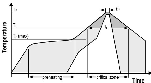
**Figure 1** Soldering profile according to JEDEC standard.  $T_P \leq 260^\circ\text{C}$  and  $t_P < 30\text{sec}$  for Pb-free assembly.  $T_L < 220^\circ\text{C}$  and  $t_L < 150\text{sec}$ . Ramp-up/down speeds shall be  $< 5^\circ\text{C}/\text{sec}$ .
