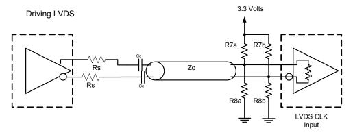
Driving LVDS inputs with the 9FGV0431
