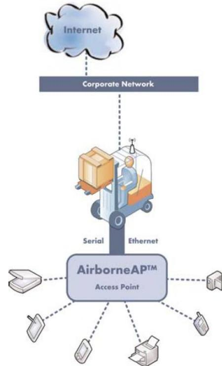
AirborneAP™ access point technology enables M2M equipment to create self sufficient Wi-Fi networks, allowing easy access to equipment data or resources from Wi-Fi-enabled devices, including laptops, tablets and handhelds powered by Android, iOS, or Windows.
