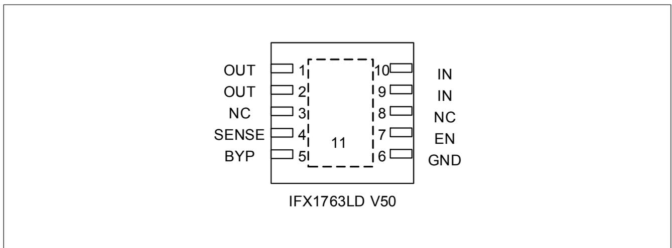
Figure 3 Pin Configuration of IFX1763LDV50 in PG-TSON10
