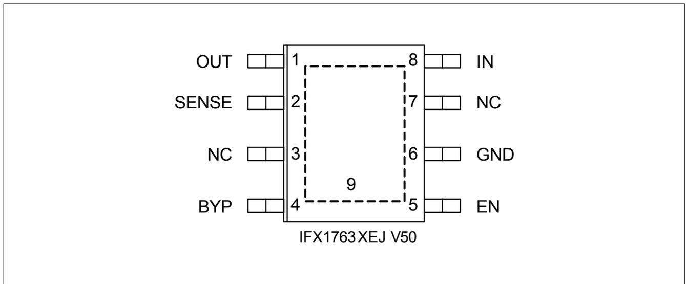
Figure 2 Pin Configuration of IFX1763XEJV50 in PG-DSO-8 Exposed Pad
