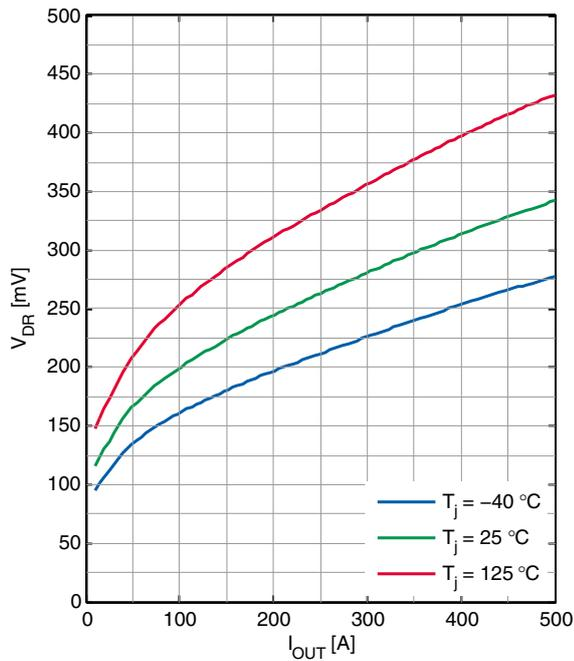
Guaranteed Dropout Voltage  $V_{DR}$  versus Output Current  $I_{OUT}$
