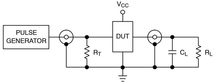
$R_T = Z_{OUT}$  of pulse generator (typically 50  $\Omega$ )
