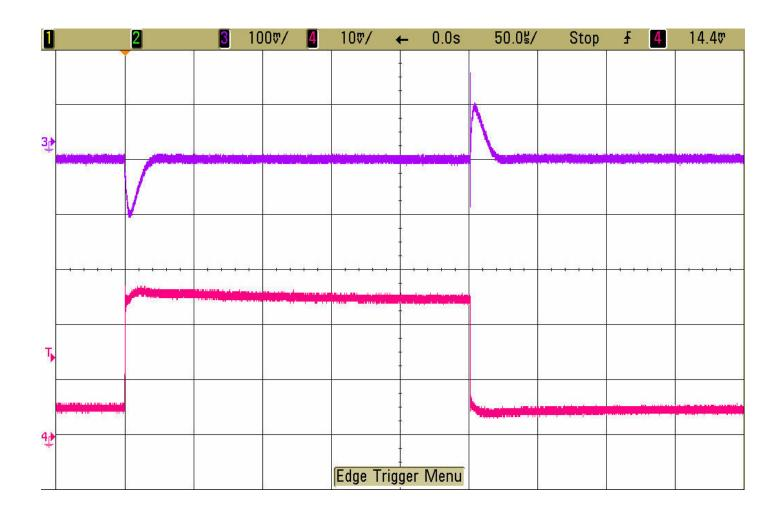
Figure 4. Load Step Response  $V_{IN} = 8.4V, V_{OUT} = 3.3V, 2A Load Step (500mA <-> 2.5A)$  Forced Continuous Mode, Fsw = 1 MHz Trace 3: Output Voltage (100mV/div AC) Trace 4: Output Current (1A/div)
