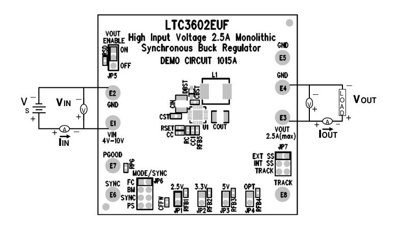
Figure 1. Proper Equipment Measurement Set-Up
