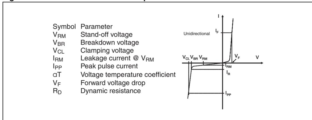
**Figure 2. Definition of  $I_{PP}$  pulse**
