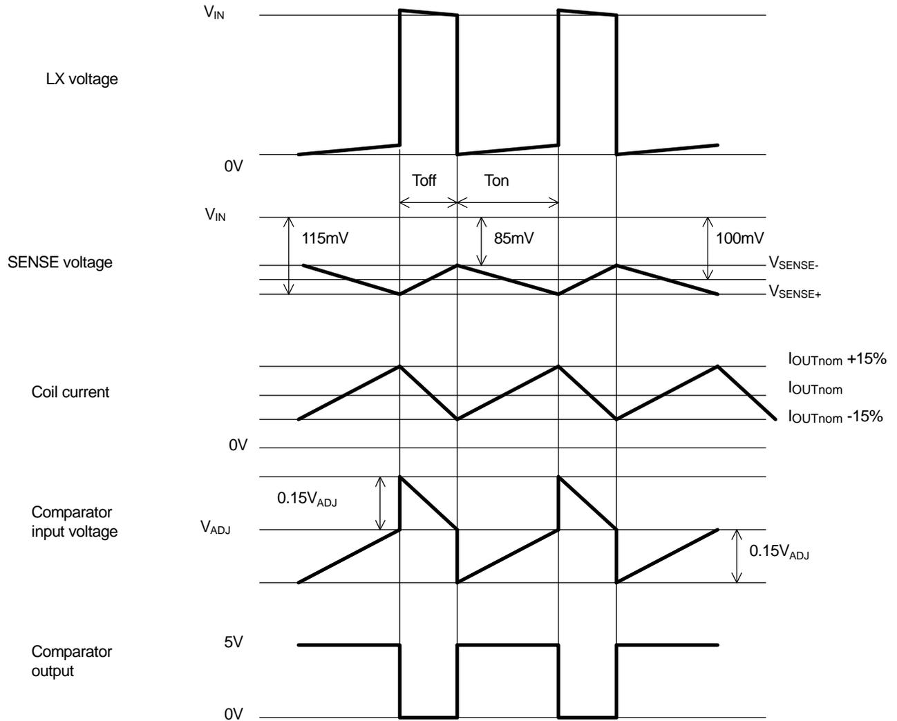
**Figure 2. Operating Waveforms**
