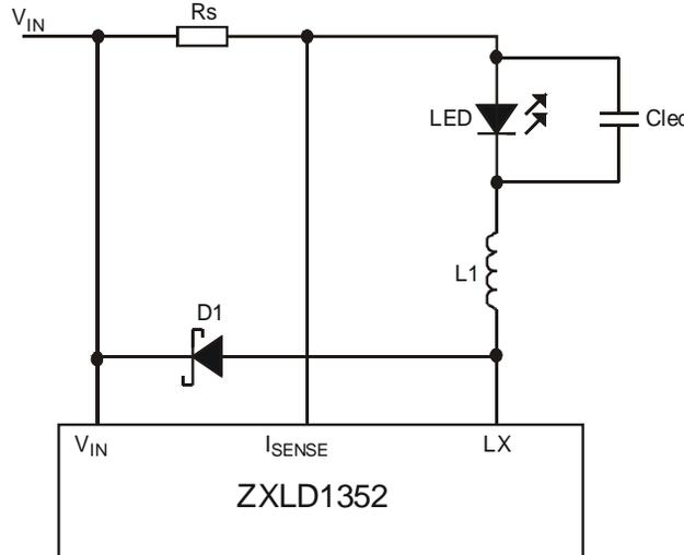
A value of  $1\mu F$  will reduce nominal ripple current by a factor three (approx.). Proportionally lower ripple can be achieved with higher capacitor values. Note that the capacitor will not affect operating frequency or efficiency, but it will increase start-up delay, by reducing the rate of rise of LED voltage.
