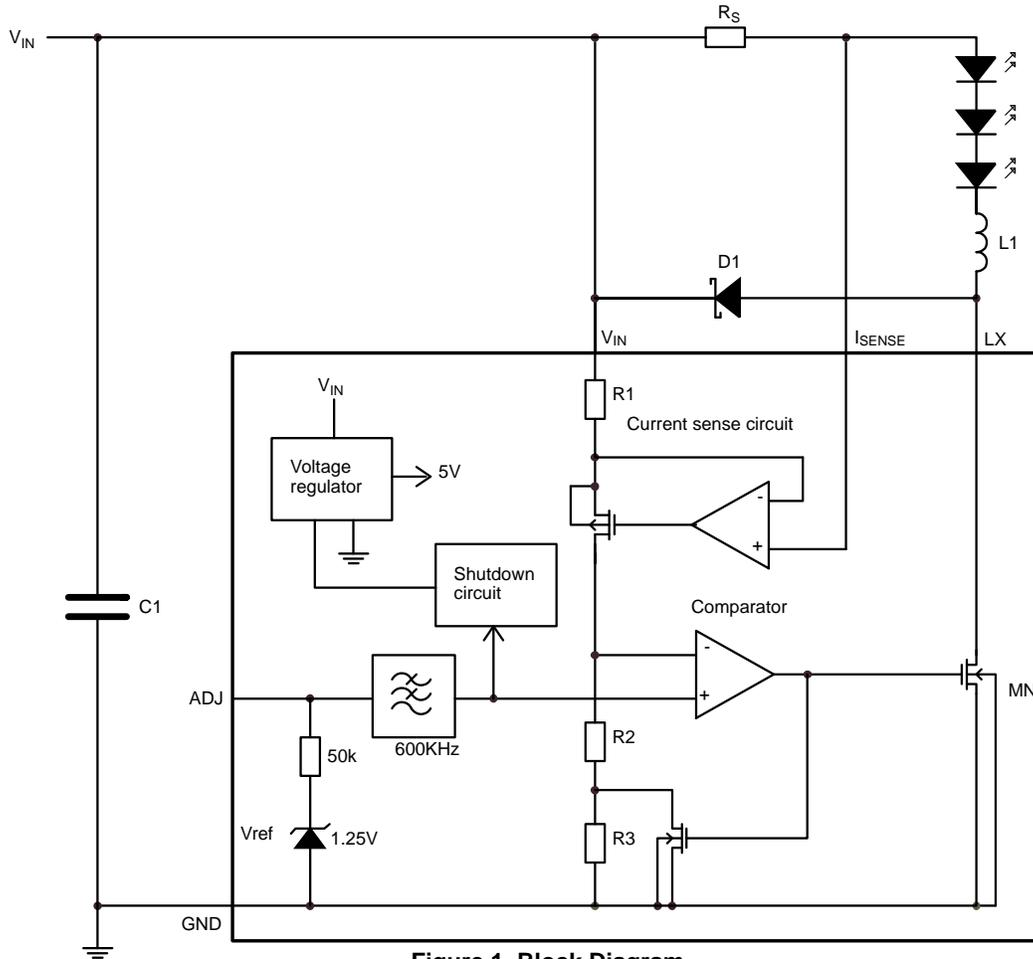
Figure 1. Block Diagram
