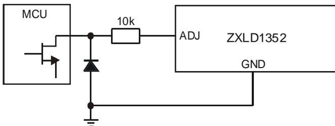
If the NMOS transistor within the microcontroller has high Gate / Drain capacitance, this arrangement can inject a negative spike into ADJ input of the ZXLD1352 and cause erratic operation but the addition of a Schottky clamp diode (eg Diodes Inc. SD103CWS) to ground and inclusion of a series resistor (3.3k) will prevent this. See the section on PWM dimming for more details of the various modes of control using high frequency and low frequency PWM signals.
