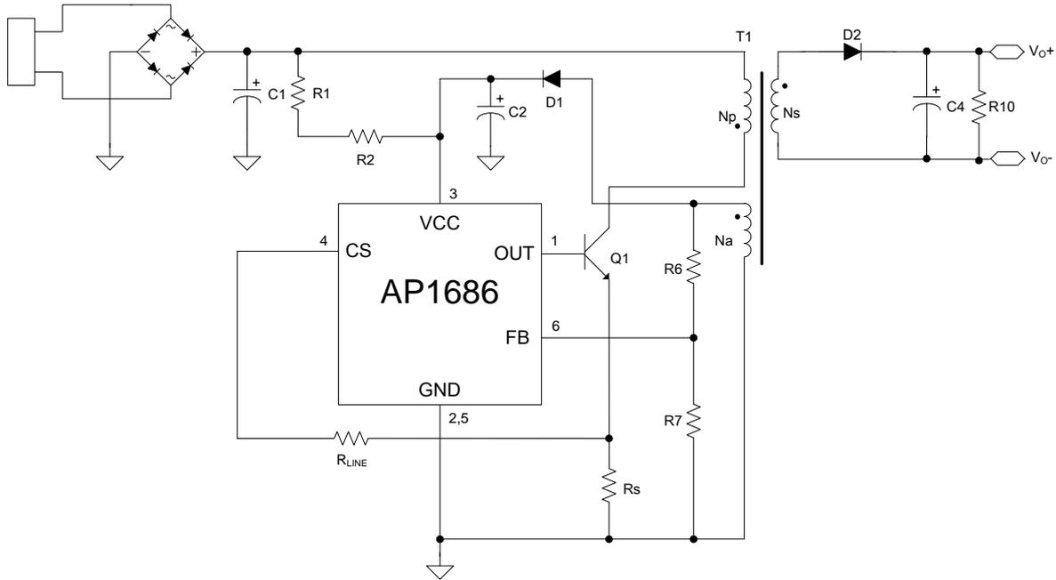
Figure 15. Typical LED Driver Application
