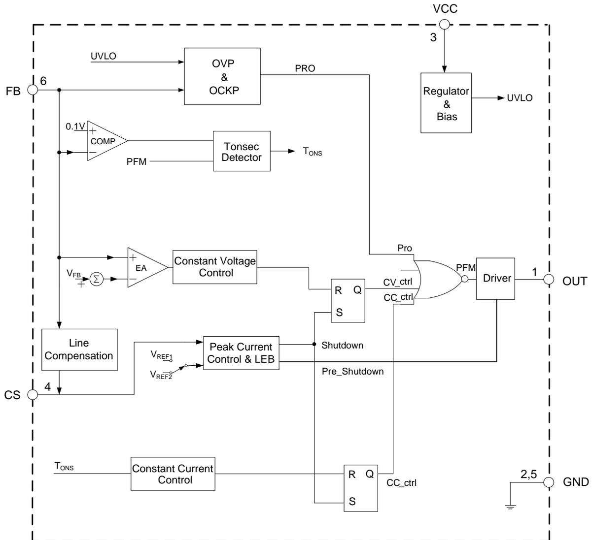
Figure 3. Functional Block Diagram of AP1686
