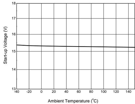
Figure 9. Start-up Voltage vs. Ambient Temperature
