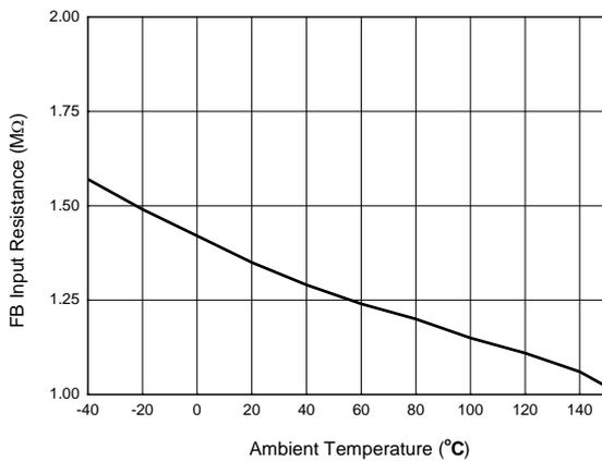
Figure 10. FB Input Resistance vs. Ambient Temperature
