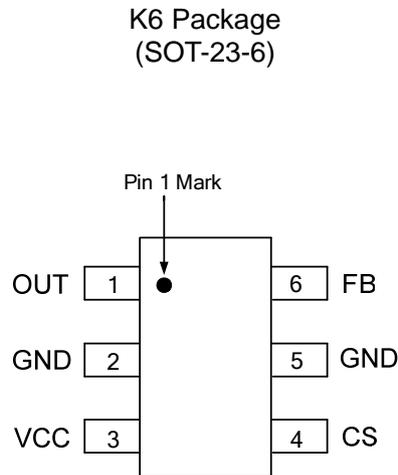
Figure 2. Pin Configuration of AP1686 (Top View)
