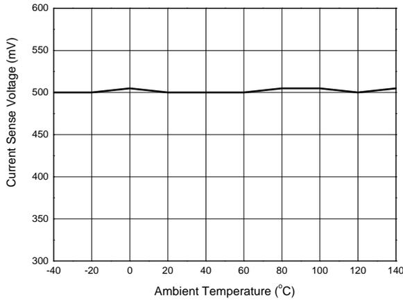
Figure 12. Current Sense Voltage vs. Ambient Temperature
