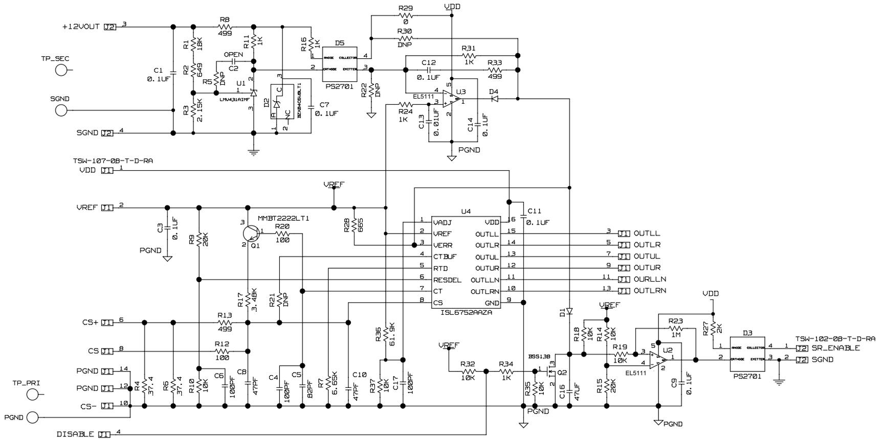
FIGURE 4. ISL6752 CONTROL CARD SCHEMATIC
