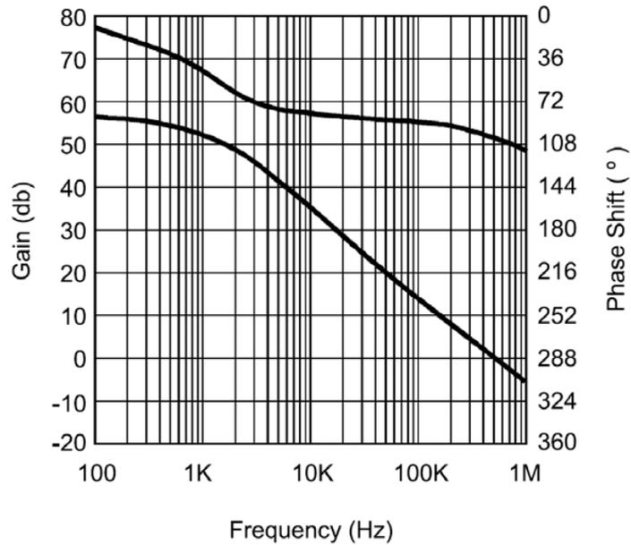
The open loop transfer function of the LMV431 is created here by inserting poles as necessary to recreate the Gain/Phase plot found in the data sheet. Note that the phase shift is relative to the input.
