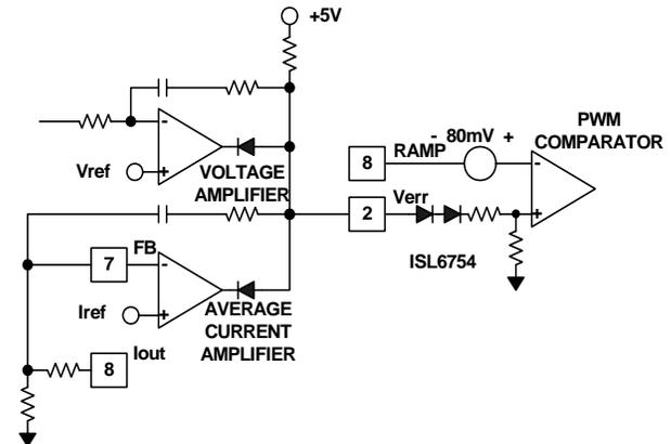
FIGURE 1. TWO AMPLIFIERS CONNECTED TO ONE PWM COMPARATOR
