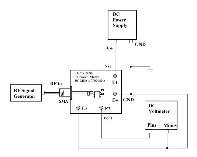
DC656A Demo Board Connection Diagram
