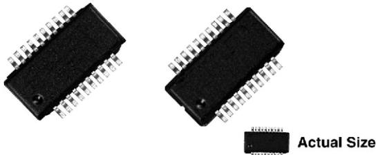
OSOP Series resistor networks feature a space saving 25 mil lead pitch versus the current 50 mil pitch standard. This allows users to reduce board space more than 50 % over current standards. The OSOP Series feature 10 isolated resistors in a 20 lead style available for immediate delivery in the standard values listed.
