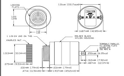
NOTE A: TERMINALS-0.32 BRASS TIN PLATED, TAPPED FOR #6-32 SCREW. TWO #6-32 NICKEL PLATED BRASS SCREWS INCLUDED. WILL ACCEPT 1/4\* QUICK CONNECT. NOTE B: MOUNTING- REMOVE BLACK PLASTIC NUT AND INSERT THREADED FRONT THROUGH 1.25' HOLE PUNCHED IN PANEL, IF DRIENTATION IS NEEDED, NOTE LOCKING FLATS ON DRAWING. SCREW NUT BACK ON. DO NOT DVERTIGHTEN.
