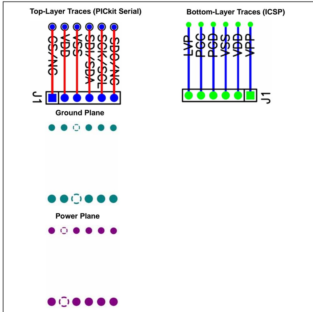
**FIGURE 2-5:** PICkit Serial / ICSP Interface Connections.
