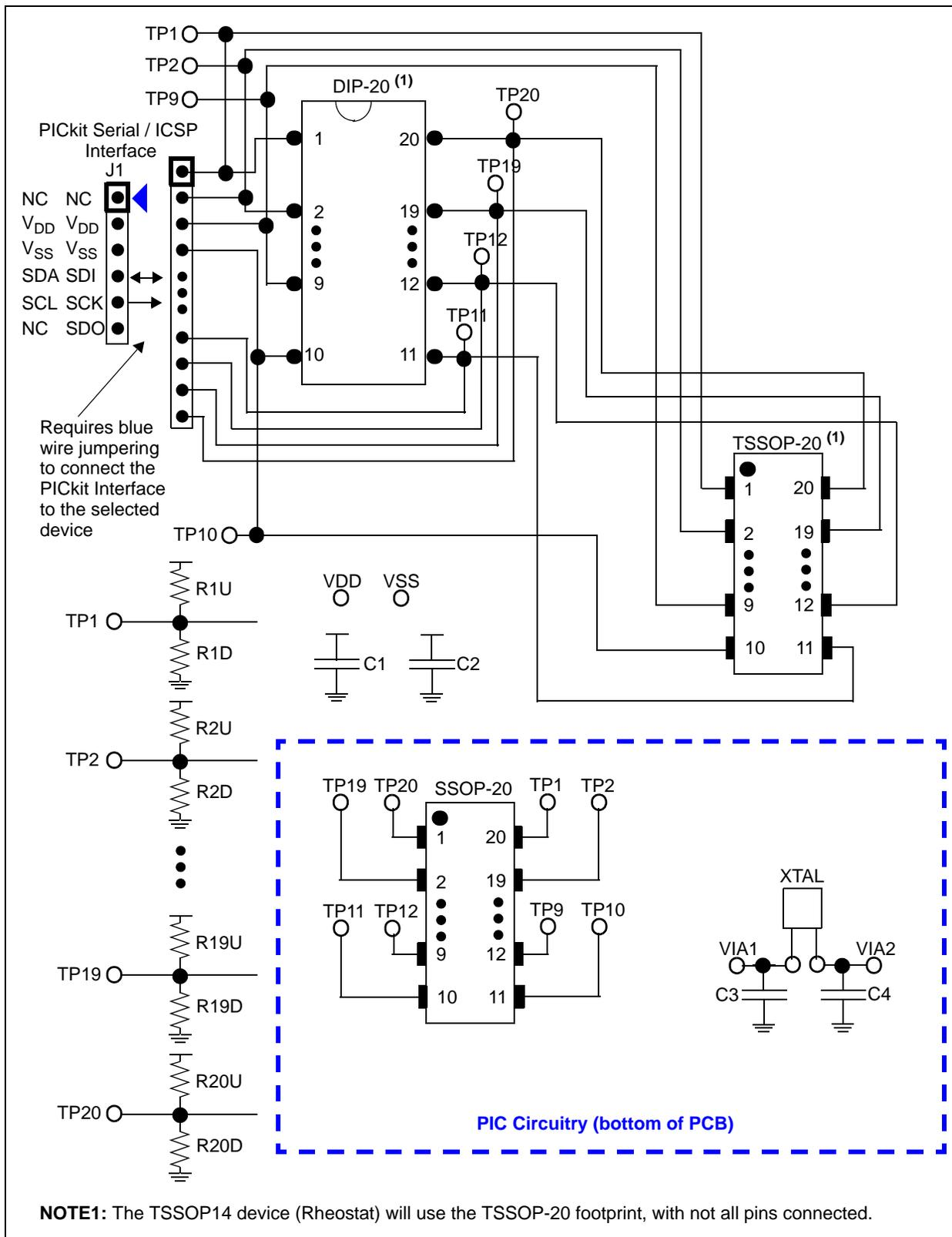
**FIGURE 2-1:** 20-Pin TSSOP and SSOP Evaluation Board Circuit.
