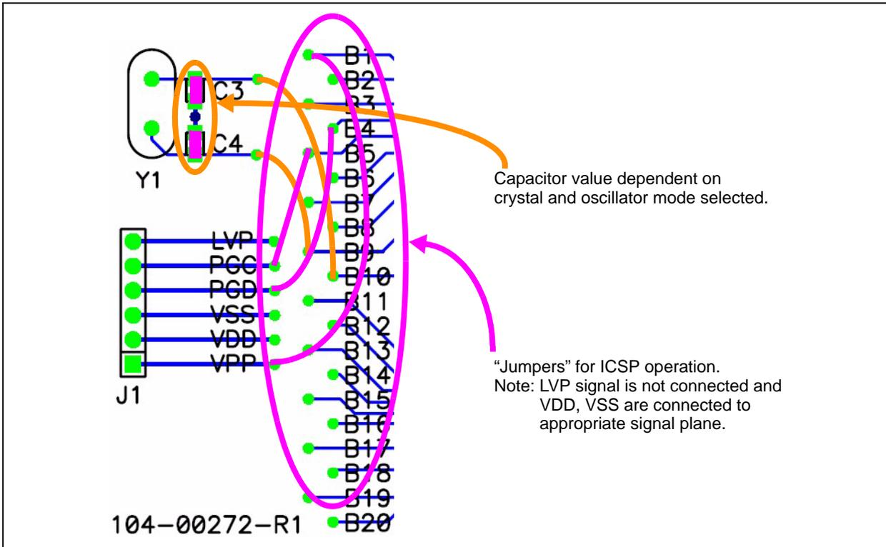
FIGURE 2-9: PIC ICSP Header Example Connections (for PIC24F16KA101).
