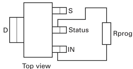
**Note:** Rprog must be connected between the Status and IN pins
