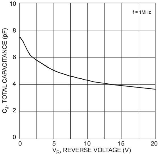
Figure 5 Typical Total Capacitance vs. Reverse Voltage
