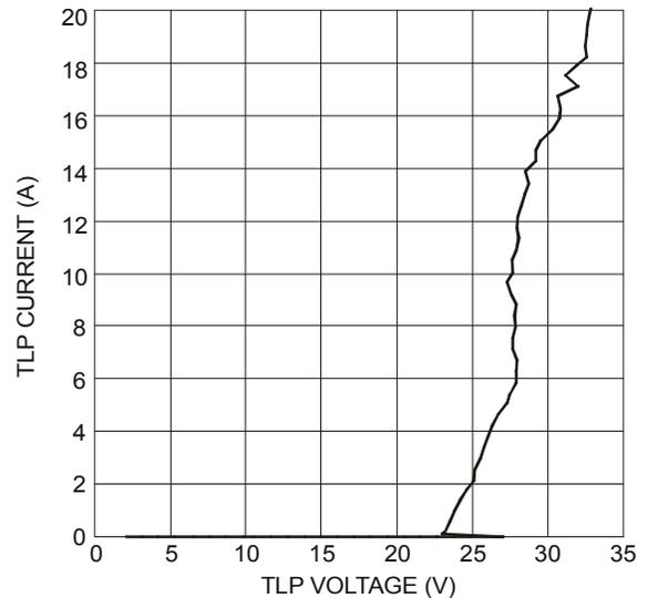
Figure 8 Transmission Line Pulsing (TLP) Current vs. Voltage
