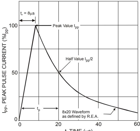
Figure 3 Pulse Waveform
