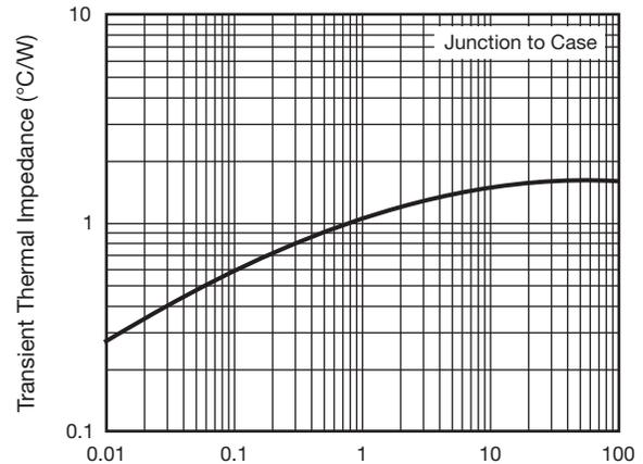
Fig. 6 - Typical Transient Thermal Impedance Per Diode
