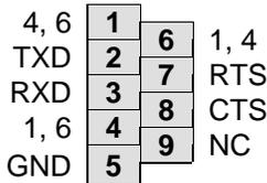
Female DB9 connector that interfaces to the MCU internal SCI0 serial port via the RS232 transceiver. Flow control is provided at test points on the board.
