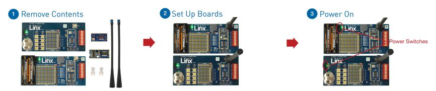
Remove the boards, antennas, batteries and connectors.
