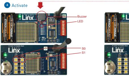
Push S0 to activate buzzer and push S1 to turn on the LED.
