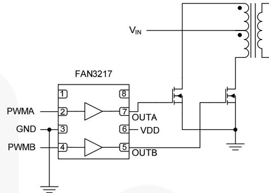
Figure 37. Primary-Side Dual Driver in a Push-Pull Converter
