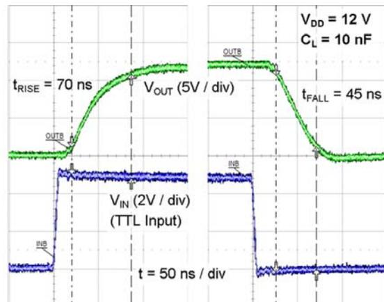
Figure 25. Rise/Fall Waveforms with 10 nF Load
