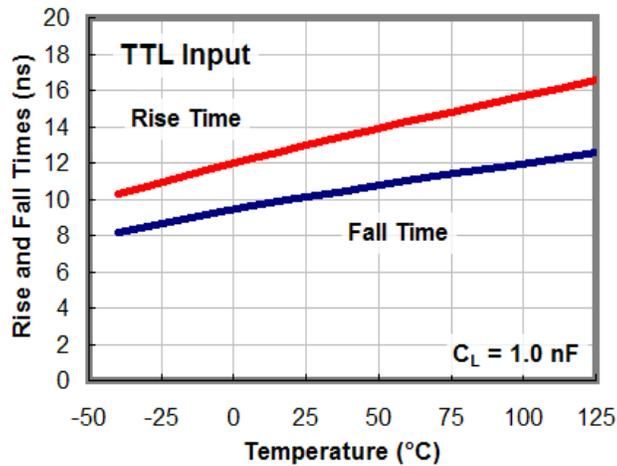
Figure 23. Rise and Fall Times vs. Temperature
