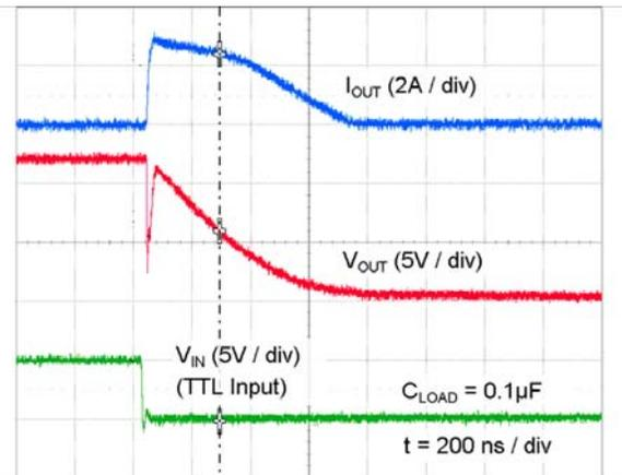
Figure 27. Quasi-Static Sink Current with  $V_{DD}=12\text{ V}$ <sup>(13)</sup>
