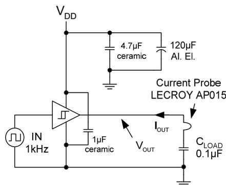
Figure 30. Quasi-Static  $I_{OUT} / V_{OUT}$  Test Circuit
