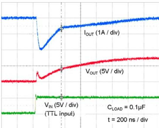
Figure 28. Quasi-Static Source Current with  $V_{DD}=8\text{ V}$ <sup>(13)</sup>
