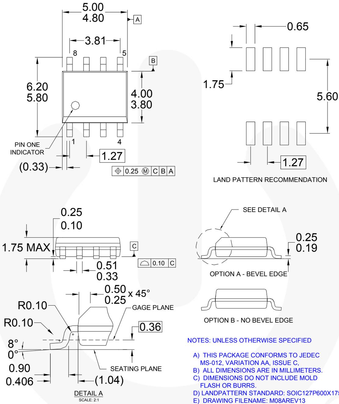
Figure 39. 8-Lead Small Outline Integrated Circuit (SOIC)
