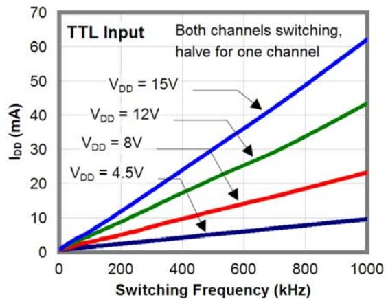
Figure 13.  $I_{DD}$  (1 nF Load) vs. Frequency
