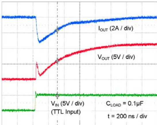
Figure 26. Quasi-Static Source Current with  $V_{DD}=12\text{ V}$ <sup>(13)</sup>
