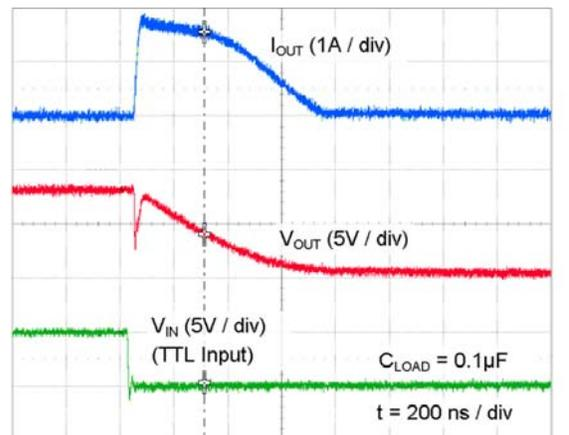
Figure 29. Quasi-Static Sink Current with  $V_{DD}=8\text{ V}$ <sup>(13)</sup>
