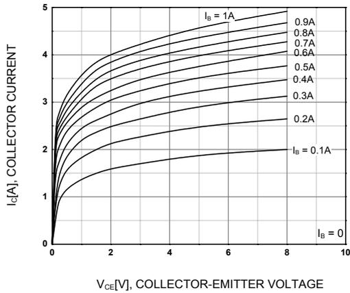
Figure 1. Static Characteristic
