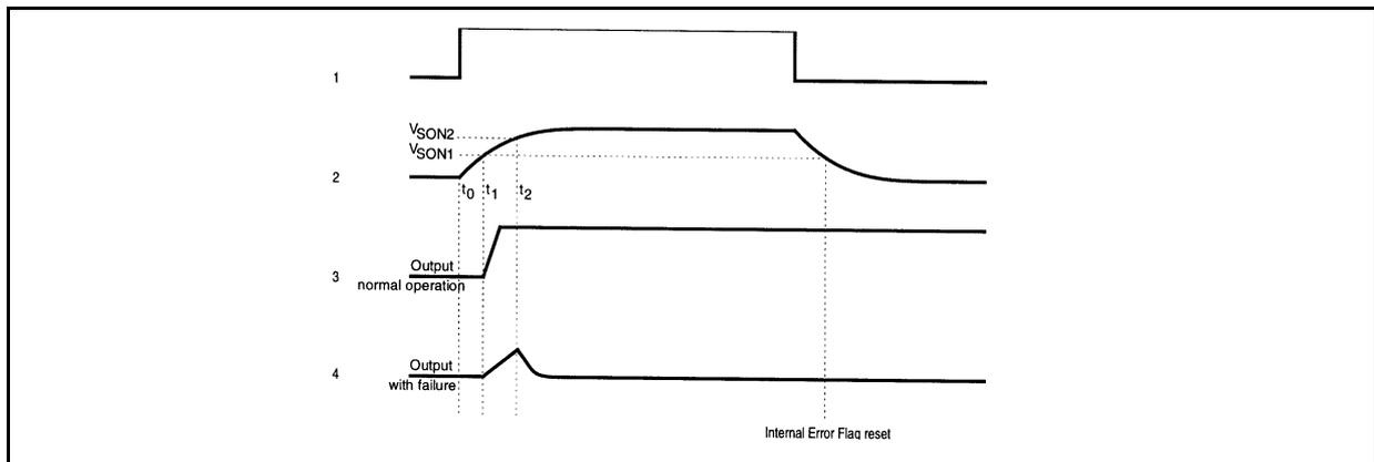
is High the device is switched on. The diagnostic circuitry detect the low drop voltage.
