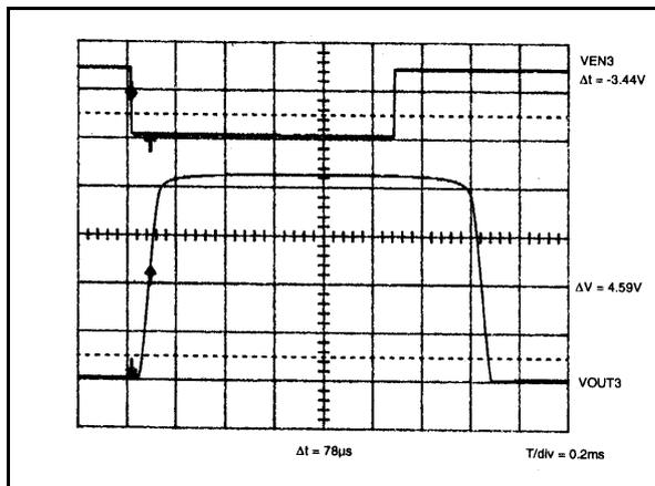
**Figure 8:** OUT1 supply transient rejection (C = 10μF, ESR = 4.7Ω, Load at OUT1 = 100Ω, Load = 10kΩ)
