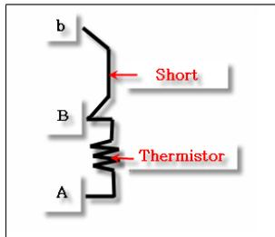
Figure 3-20 ADAM-4015T Thermistor Input Module Wiring Diagram
