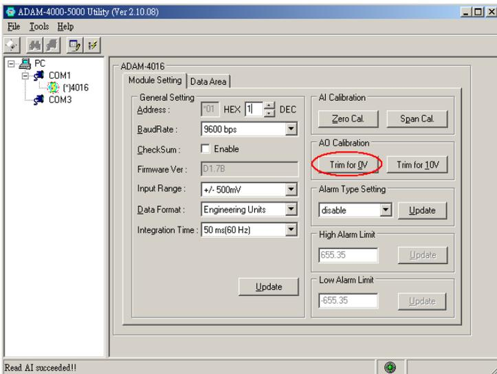
**Figure 8-8 Zero Calibration**
