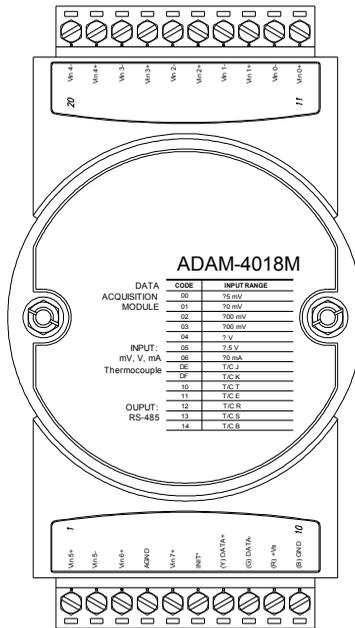
**Figure 3-28 ADAM-4018M 8-channel Analog Input Data Logger**
