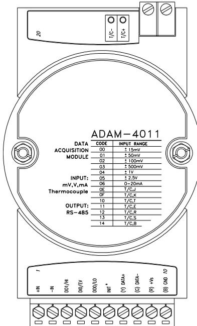
Figure 3-1 ADAM-4011 Thermocouple Input Module
