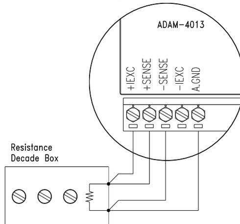
**Figure 8-5** Applying calibration resistance
