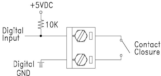
**Figure 3-8 ADAM-4011/4011D Digital Input Wiring Diagram
