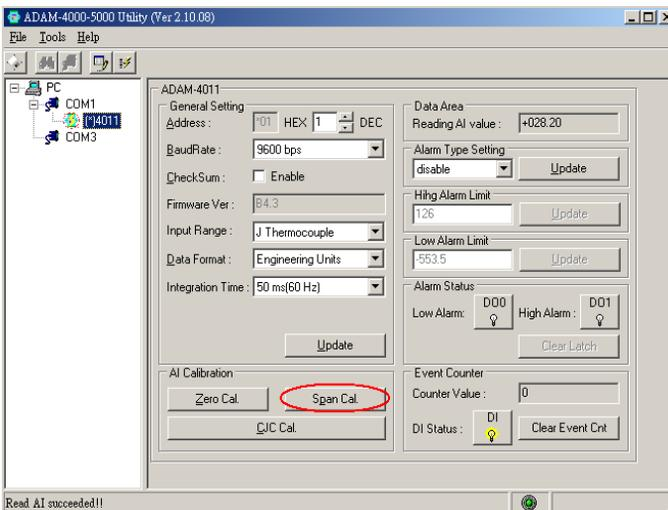
**Figure 8-3 Span Calibration**
