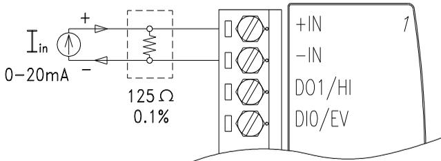
Figure 3-11 ADAM-4012 Process Current Input Wiring Diagram
