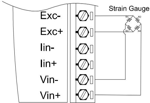
Figure 3-22 ADAM-4016 Strain Gauge Voltage Input Wiring Diagram
