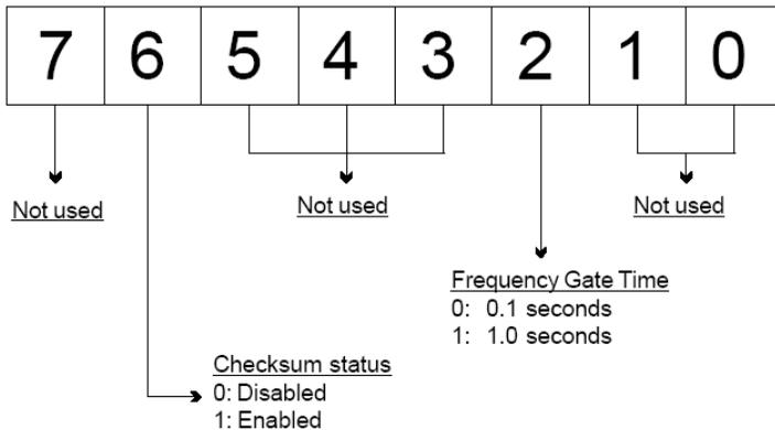
**Figure 7-3 Data format for FF (8-bit parameter)**
