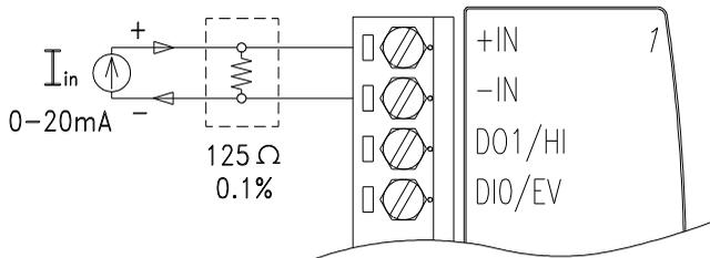
Figure 3-5 ADAM-4011/4011D Process Current Input Wiring Diagram
