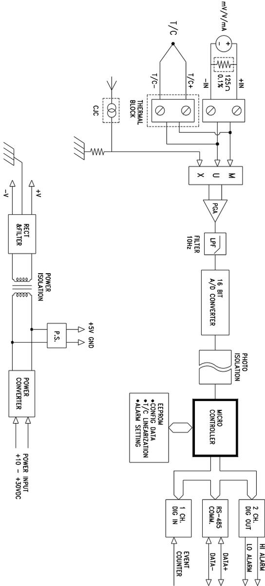
**A.2 ADAM-4011D Thermocouple Input Module with LED Display**
