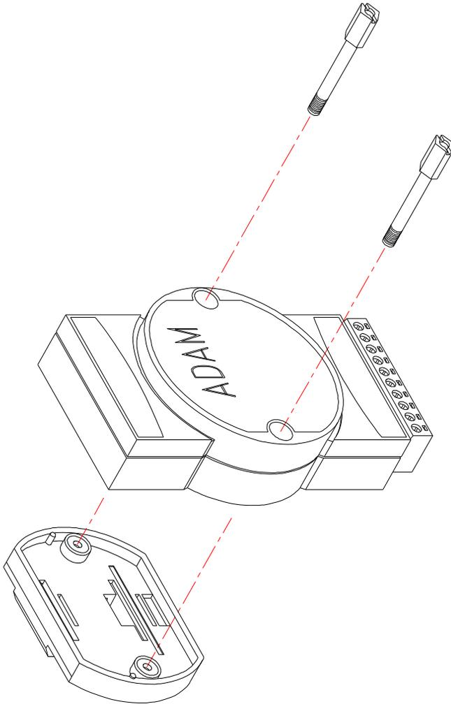
**Figure C-2** *DIN-Rail Adapter*
