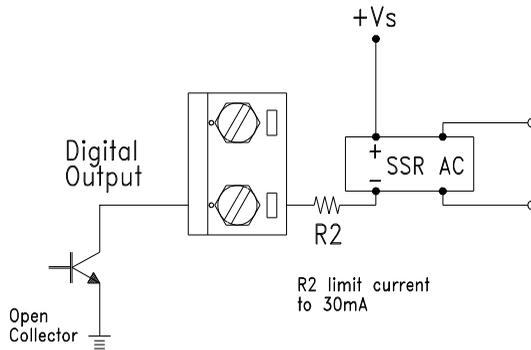
Figure 3-12 ADAM-4012 Digital Output Wiring Diagram
