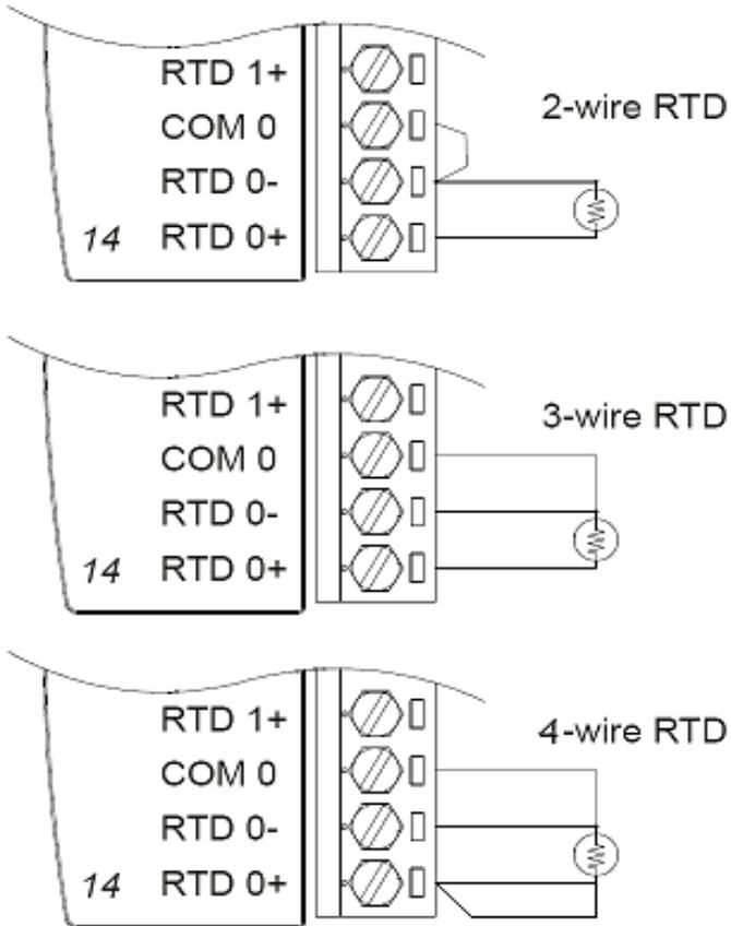
Figure 3-18 ADAM-4015 RTD Input Module Wiring Diagram
