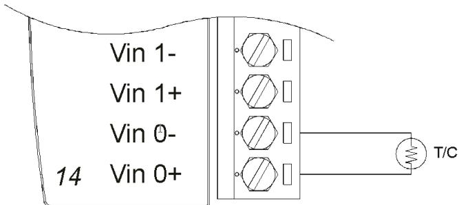
Figure 3-35 ADAM-4019+ Universal Analog Input Wiring Diagram
