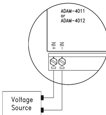
**Figure 8-1** *Applying Calibration Voltage*
