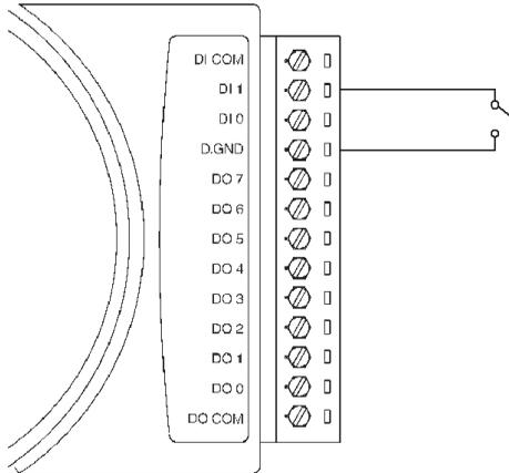
Figure 3-54a ADAM-4055 Digital Input Dry Contact Wiring Diagram
