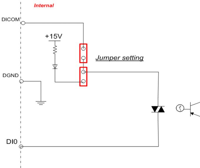
**Figure 3-56a ADAM-4055 Default Jumper Setting for the Digital Input Wiring
