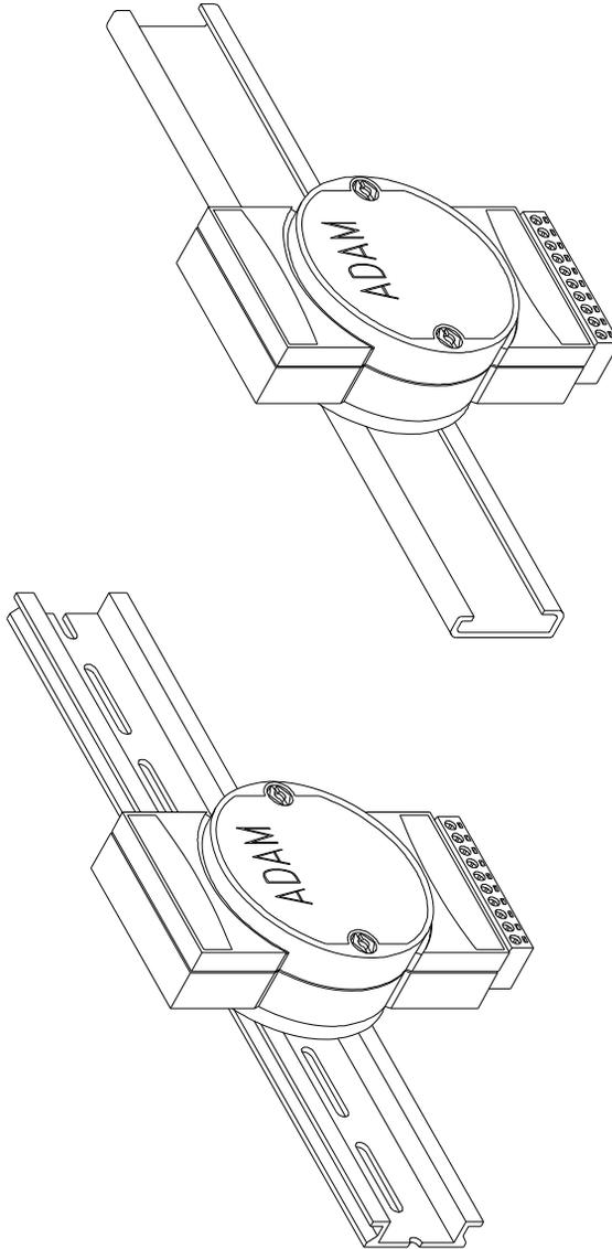
**Figure C-3 DIN-Rail Mounting**
