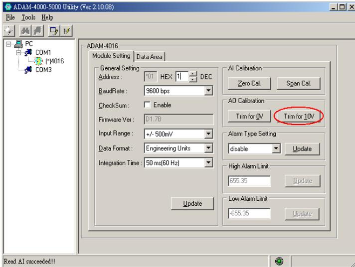
**Figure 8-9 Span Calibration**
