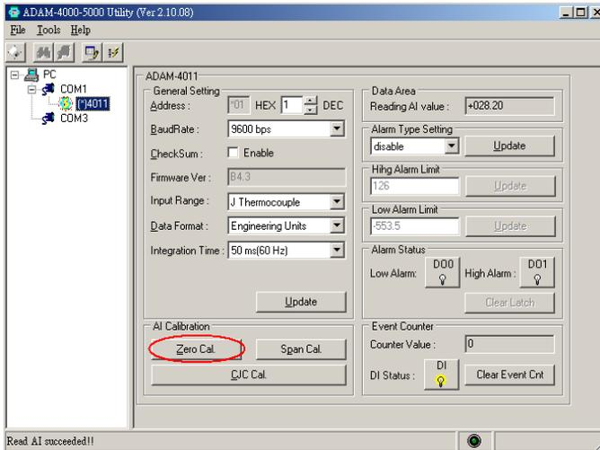
**Figure 8-2 Zero Calibration**
