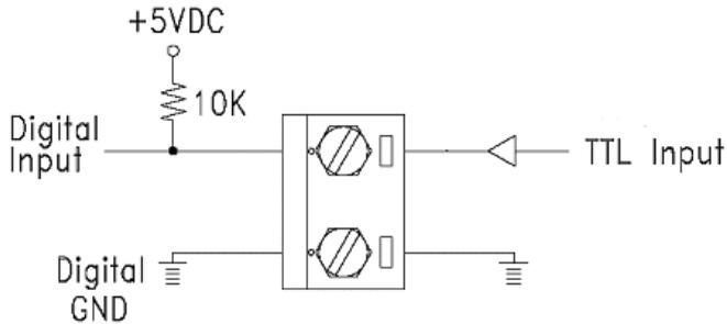
**Figure 3-7 ADAM-4011/4011D Digital Input Wiring Diagram
