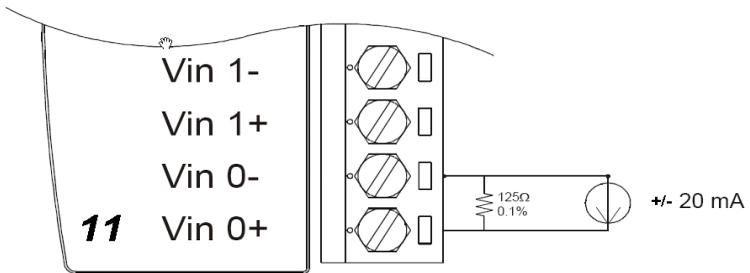
**Figure 3-30 Current Input Wiring Diagram of ADAM-4017**
