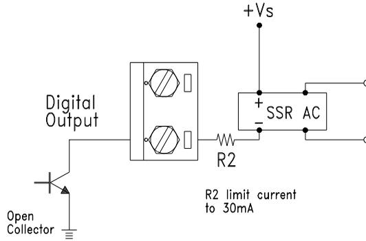
**Figure 3-6 ADAM-4011/4011D Digital Output Wiring Diagram
