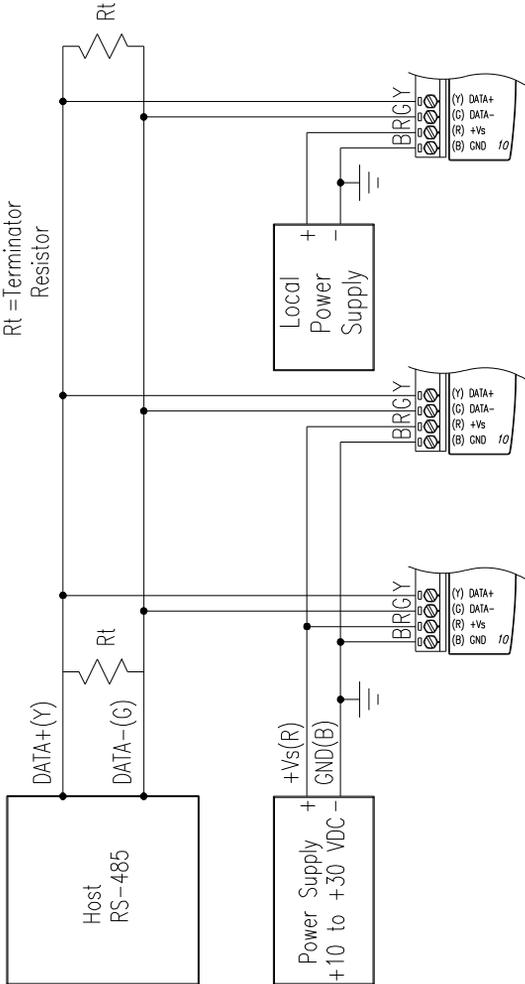
Figure 2-5 Multi-module Connection
