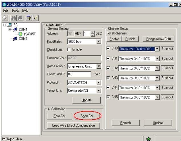
7. Apply 30K ohm's resistor with 0.01 % accuracy to CH0 and then Click on “Save”
