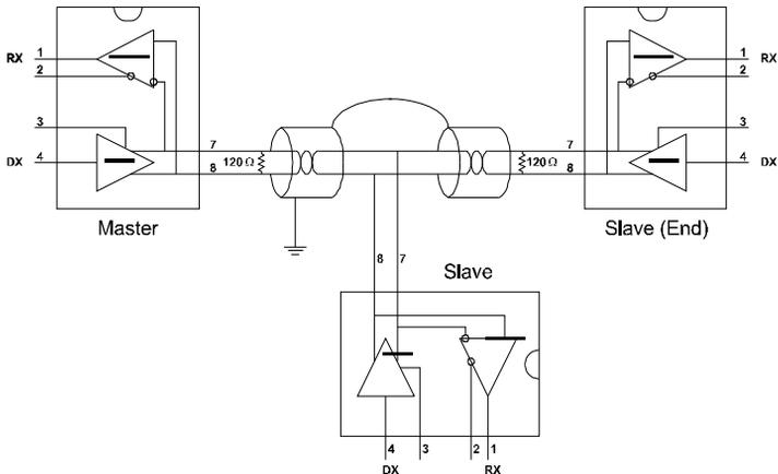
**Figure E-5 Termination resistor locations**
