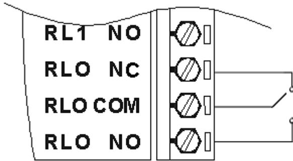
**Figure 3-65 ADAM-4068 Form C Relay Output Wiring Diagram**
