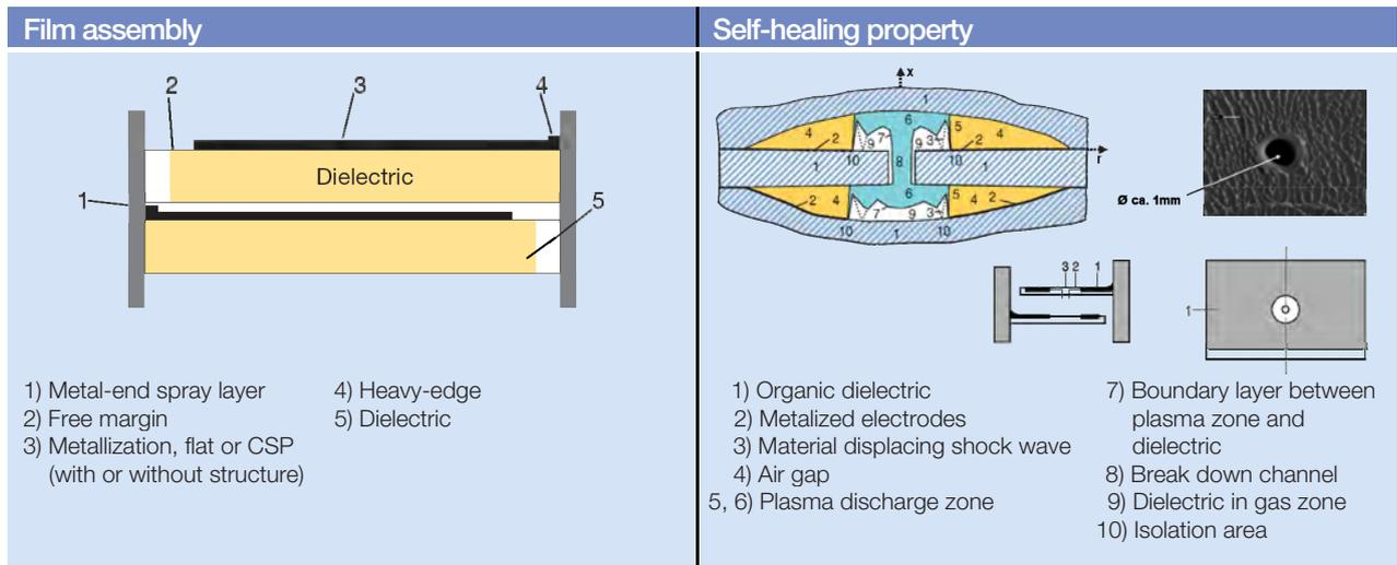
Fig. 1: Cross section of a metalized film capacitor
