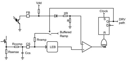
Figure 36. Ramp Compensation Setup
