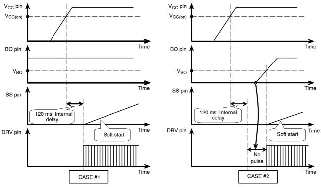
Figure 30. Different Startup Sequence Case #1 & #2
