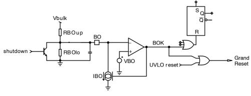
Figure 34. BO Pin Setup
