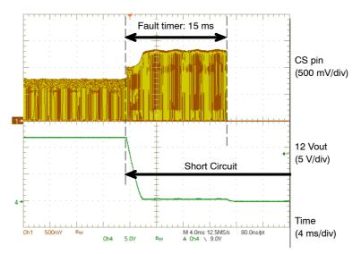
Figure 35. Short Circuit Detection Example
