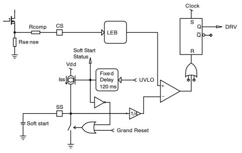
Figure 32. Soft Start Principle
