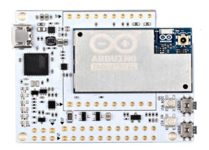
The Arduino Industrial 101 is a break-out board for the Arduino 101 LGA module. Just like the YUN, it integrates an ATmega32U4 and an Atheros AR9331 with WiFi and Linino OS.
