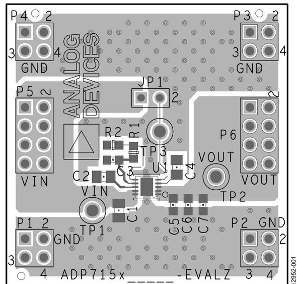
Figure 1. **ADP7157CP-04-EVALZ** Printed Circuit Board (PCB) Layout
