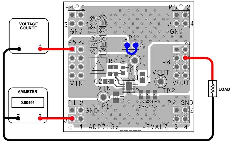
Figure 7. Ground Current Measurement Setup for the [ADP7157CP-04-EVALZ](#)
